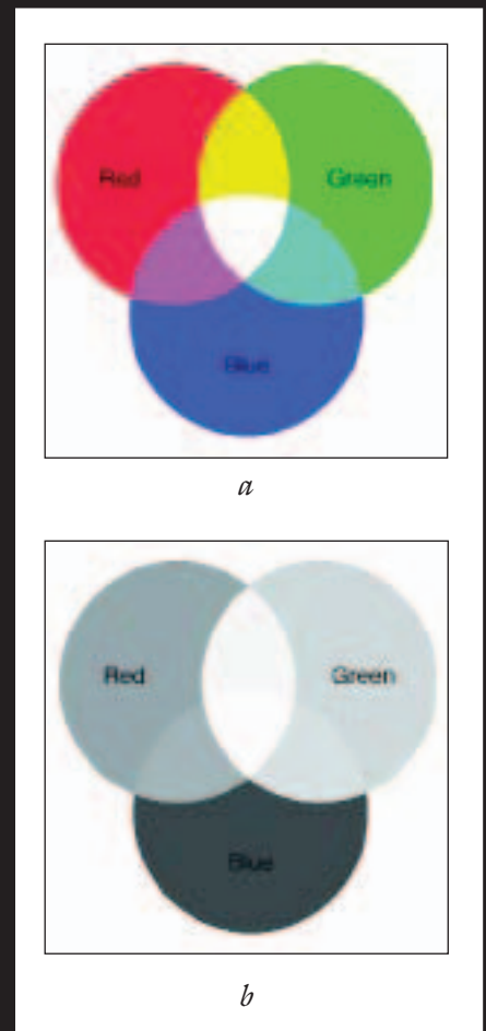
FIGURES 4-2A AND B. COLOR WHEEL. (a) RGB Color. (b) Grayscale conversion.
